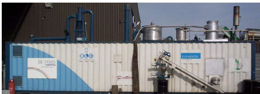
50 kg/h leather wastes containerised gasifier coupled with gas cleaning system
